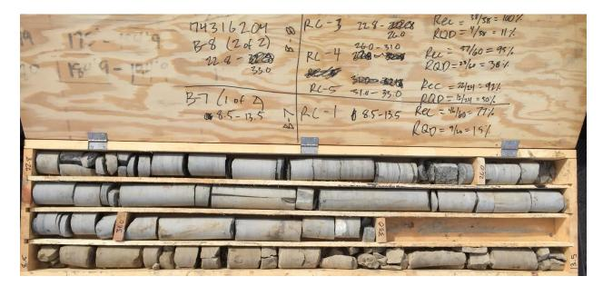
Photo 9B-8, Run 3 through Run 5 (22.8'-33.0'), Box 2 of 2B-7, Run 1 (8.5'-13.5'), Box 1 of 2
