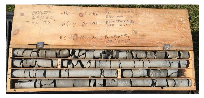
Photo 11 B-9, Run 1 through Run 3 (13.0'-28.0'), Box 1 of 2
