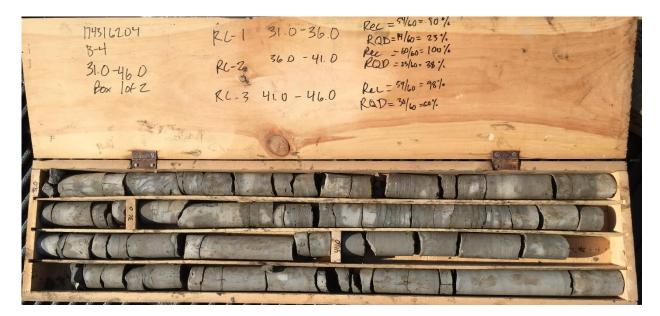
Photo 4 B-4, Run 1 through Run 3 (31.0'-46.0'), Box 1 of 2
