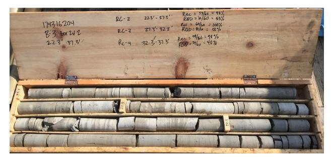
Photo 3 B-3, Run 2 through Run 4 (22.3'-37.3'), Box 2 of 2
