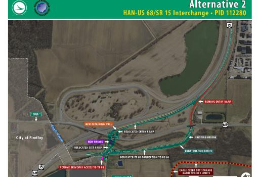
Alternative 2: Provides a dedicated connection of Township Road 80 to U.S. 68. A new bridge would be constructed over Eagle Creek and a new retaining wall for the new entry ramp to State Route 15.
