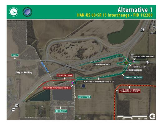
Alternative 1: Includes a dedicated connection from Township Road 80 to U.S. 68 with a single lane roundabout. The relocated east bound exit ramp will also connect to the new roundabout.
