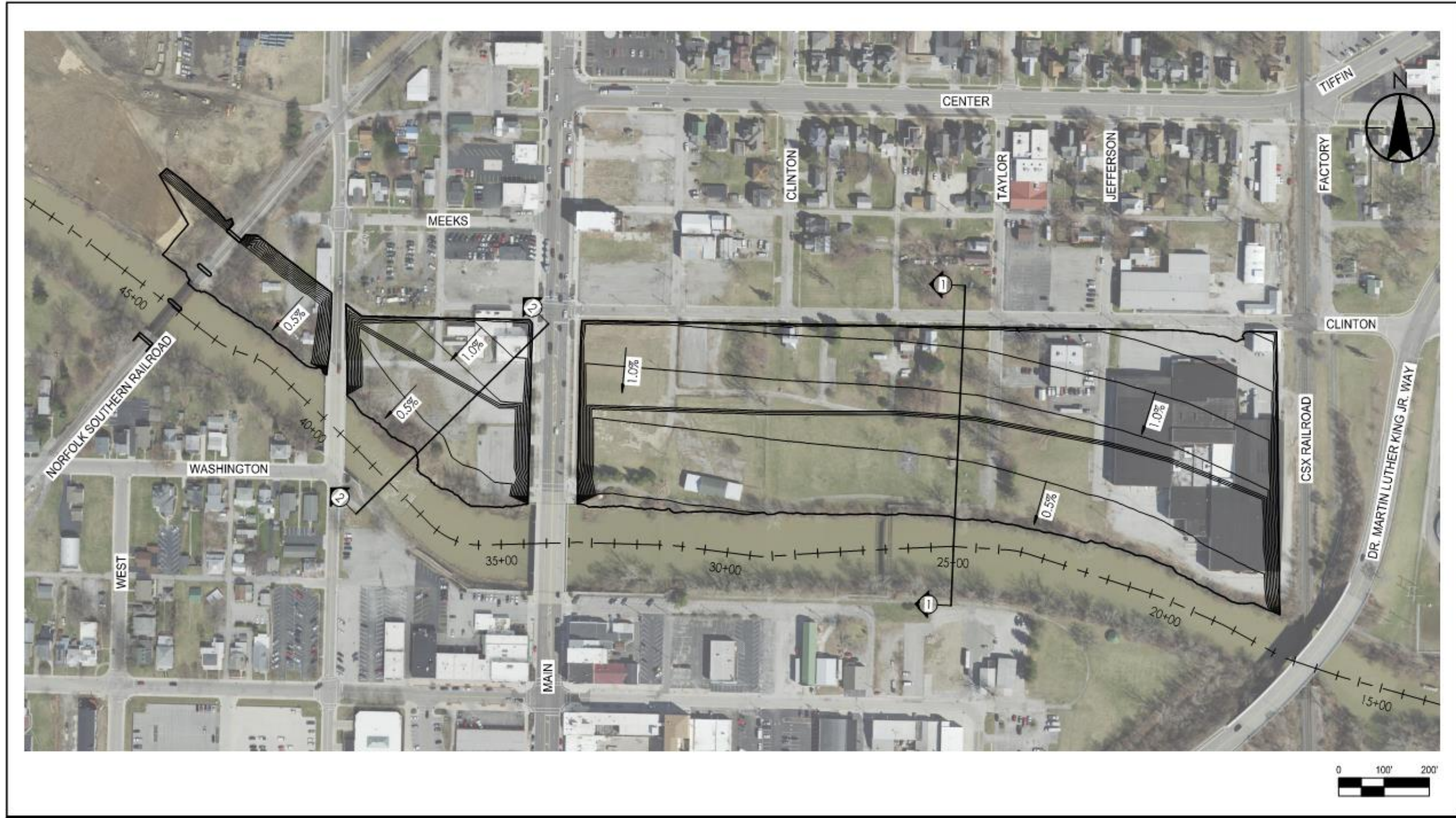
Figure 10 – Preliminary Design Concept 2 – Plan View
